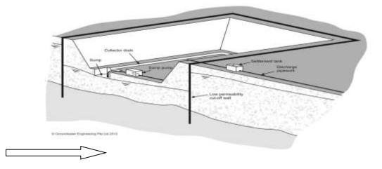
In this method, low permeability cut off wall is constructed along the area of excavation and further pumps are installed in such a way that the water collected to cut off walls can be pumped and collected in a tank.
