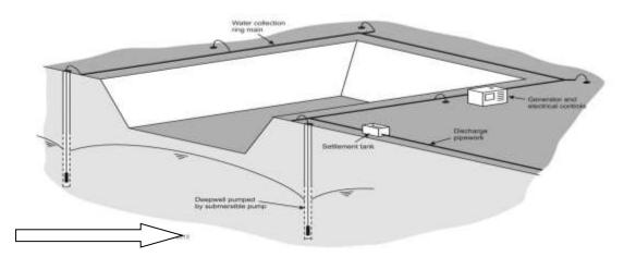
1)Dewatering can draw groundwater levels down to elevations not impacted by construction through pumping wells and/or a connected well point system.2) A thorough understanding of the underlying soils and groundwater conditions is required to develop this type of design input.
